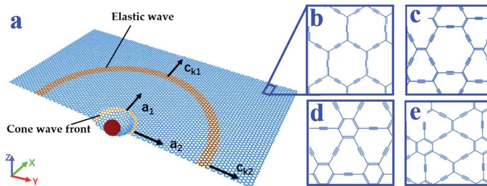
Fig. 1 (a) Schematic diagram of the impact. The yellow and orange rings represent the positions where the cone wave front and elastic wave propagate to, respectively. Structures of (b)  $\alpha$ -graphyne, (c)  $\beta$ -graphyne, (d)  $\delta$ -graphyne, and (e)  $\gamma$ -graphyne.
