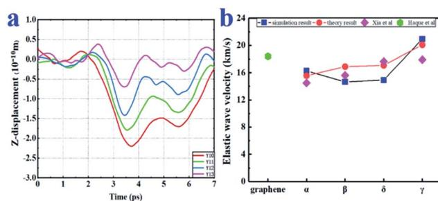
Fig. 2 (a) Displacement–time plots in the  $Y$ -direction (points Y10–Y13) for  $\alpha$ -graphyne under a  $2.0 \text{ km s}^{-1}$  impact. (b) Comparison of the theoretical and simulated values of elastic wave propagation velocity in the  $X$  direction. The simulated values of both Haque *et al.*<sup>10</sup> and Xia *et al.*<sup>34</sup> are shown for comparison.
