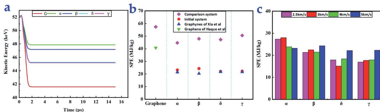
**Fig. 4** (a) Change in kinetic energy over time for a projectile impacting graphynes and graphene (red line) at an impact velocity of  $5 \text{ km s}^{-1}$  (b) SPE values of graphynes and graphene for a  $5 \text{ km s}^{-1}$  impact velocity along with corresponding values from Haque *et al.*<sup>10</sup> and Xia *et al.*<sup>34</sup> (c) SPE values of the initial systems for different impact velocities from  $2.5$  to  $5 \text{ km s}^{-1}$ .
