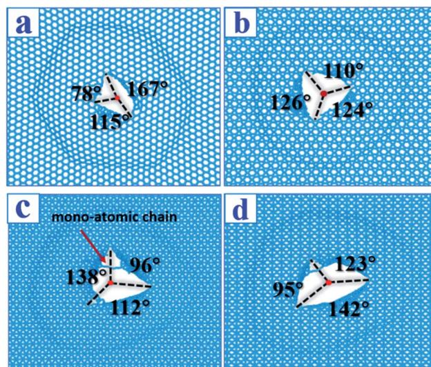
Fig. 5 Comparisons between our room temperature fracture patterns and low temperature patterns (Xia) after impact for graphynes. Impact velocity is  $2.5 \text{ km s}^{-1}$ . The left line is our patterns, the right is from Xia *et al.*<sup>34</sup> (a)  $\alpha$ -Graphyne; (b)  $\beta$ -graphyne; (c)  $\delta$ -graphyne; (d)  $\gamma$ -graphyne. For whole penetration process, please see ESI videos.†
