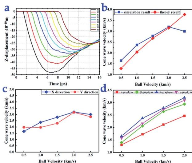
**Fig. 3** (a) Displacement–time diagram in the Z-direction (points Y10–Y13) for  $\alpha$ -graphyne under a  $2.0 \text{ km s}^{-1}$  diamond projectile impact. (b) Comparison of the theoretical and simulated values of  $\delta$ -graphyne cone wave velocity in the X direction. (c)  $\delta$ -Graphyne cone wave propagation velocities in the X and Y directions. (d) Cone wave propagation velocity in the X direction as a function of ball velocity.
