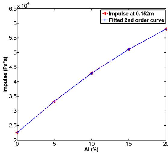
Fig. 11. Variation of impulse with mass fraction of aluminum.
