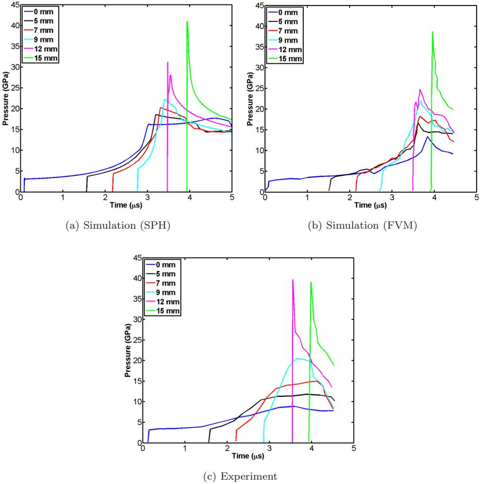
Fig. 4. Comparison of simulation with FVM and experiment.
