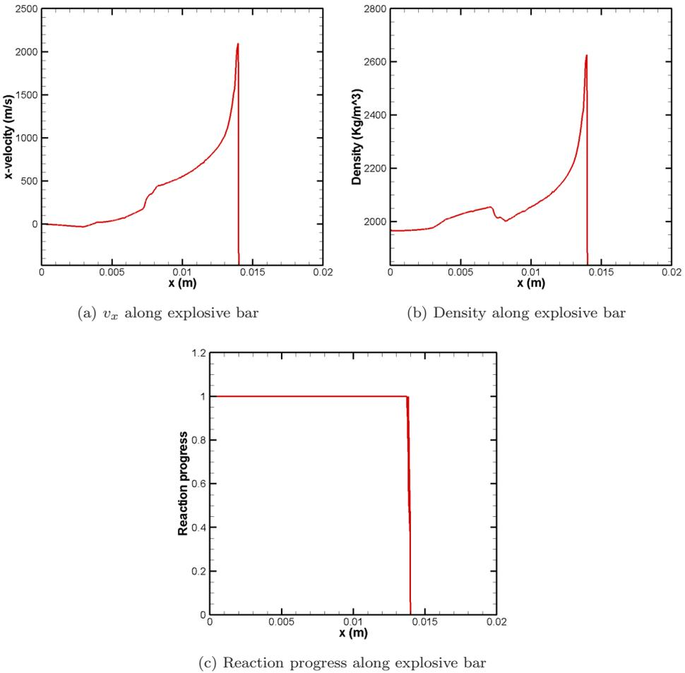
Fig. 3. Distribution of velocity, density and reaction progress along the explosive bar at  $3.5 \mu\text{s}$ .
