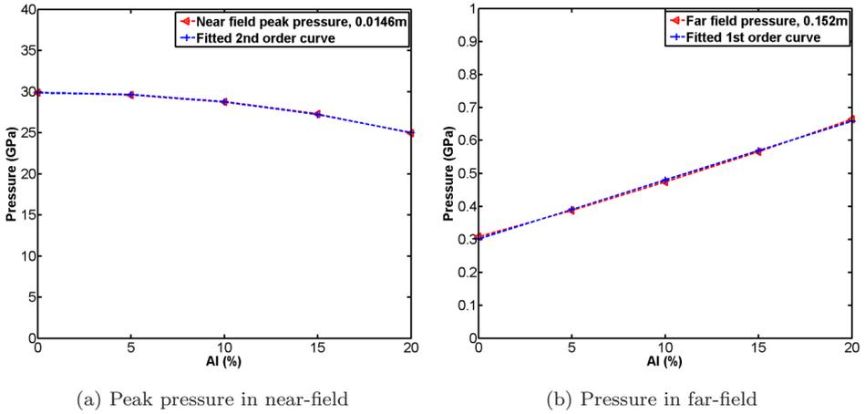
Fig. 10. Variation of pressure with mass fraction of aluminum.
