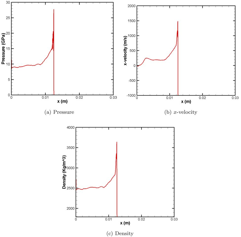
Fig. 7. Distribution of pressure,  $x$ -velocity and density along the aluminized explosive bar.
