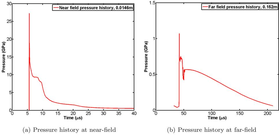
Fig. 8. Pressure history of HMX–Al at near-field and far-field.
