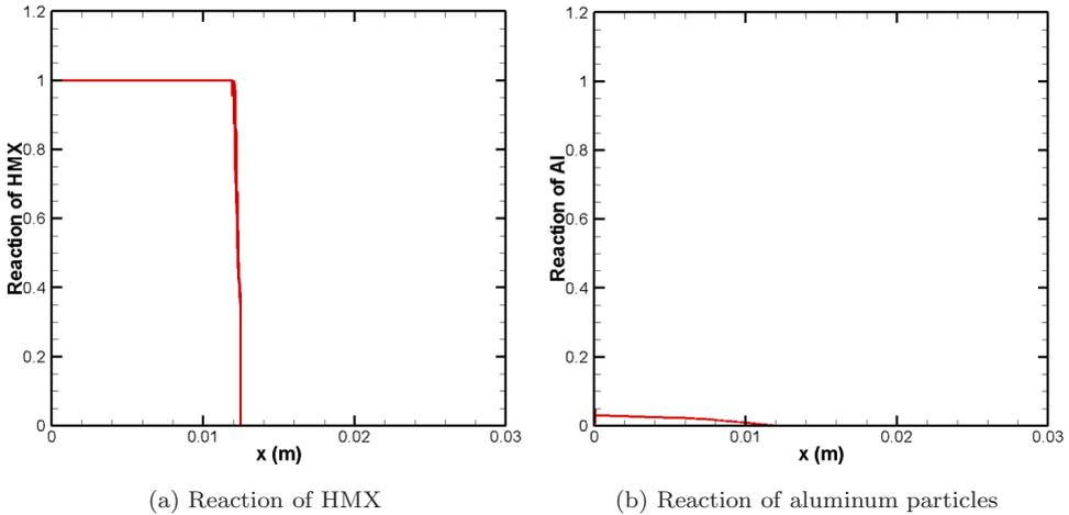
Fig. 6. Comparison of reaction progress of HMX and aluminum particles.
