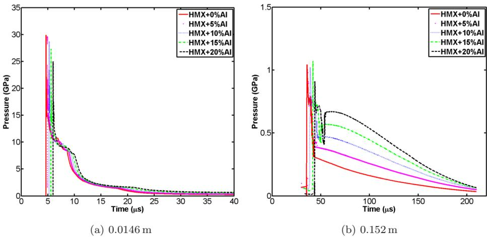
Fig. 9. Influence of mass fraction of aluminum on pressure history at near-field and far-field.
