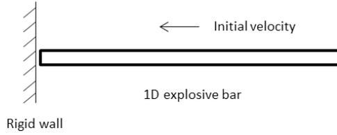
Fig. 1. 1D model of PBX 9501 bar.
