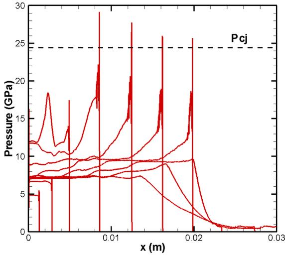
Fig. 5. Evolution of pressure along the aluminized explosive bar. Each curve represents distribution of pressure at specific time. From left to right, there are 10 curves in total and the time is from  $1 \mu\text{s}$  to  $10 \mu\text{s}$ .
