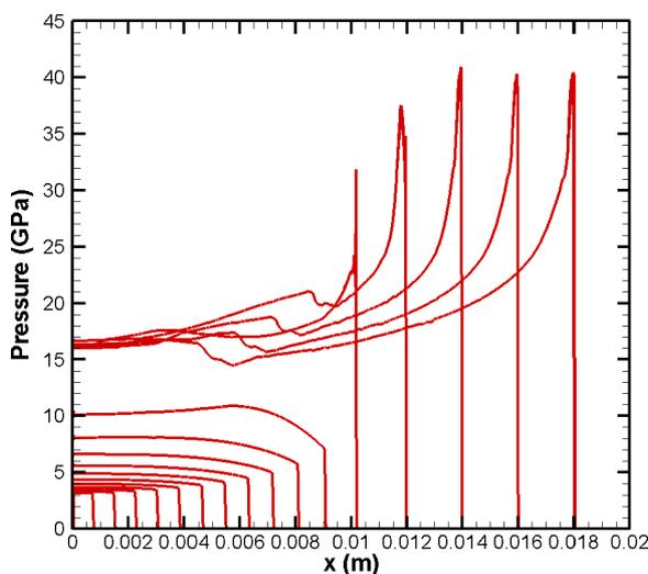
Fig. 2. Variation of shock wave. Each curve represents the distribution of pressure along the explosive bar at specific time.
